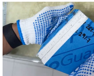
ProGuard vs Cement Board after 7 days full immersion in water
