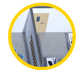
65 dB Range Classroom to a Music Room with 30m 2 dividing partition / 5dB correction factor
